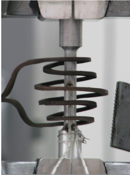
Fig. 5 Aluminum alloy AlCu4Mg1 tensile specimen with a two spot welded thermocouple.
