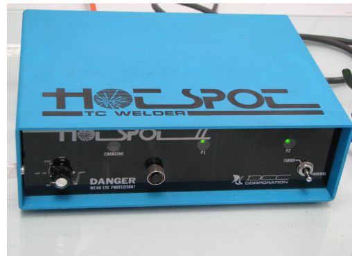
Fig. 3 HotSpot II thermocouple welder
