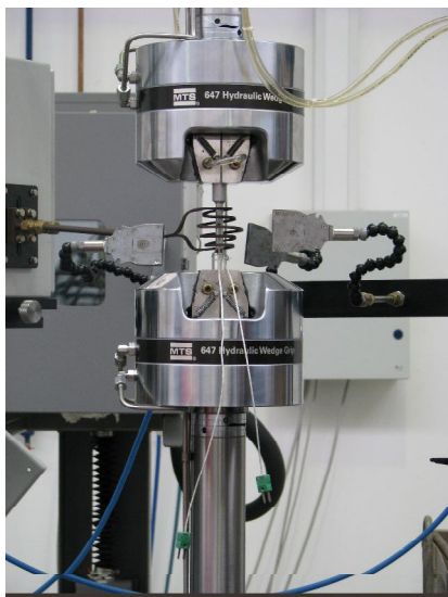
Fig. 1 MTS 810 Material test system.
