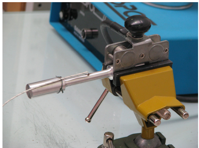
Fig. 4 Aluminium alloy tensile specimen with a spot welded thermocouple in the middle of the sample.
